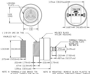
NOTE A: TERMINALS-032 BRASS TIN PLATED, TAPPED FOR #6-32 SCREW. TWO #6-32 NICKEL PLATED BRASS SCREWS INCLUDED. WILL ACCEPT 1/4' QUICK CONNECT. NOTE B: MOUNTING- REMOVE BLACK PLASTIC NUT AND INSERT THREADED FRONT THROUGH 1.25' HOLE PUNCHED IN PANEL, IF DRIENTATION IS NEEDED, NOTE LOCKING FLATS ON DRAWING, SCREW NUT BACK ON. DO NOT OVERTIGHTEN.
