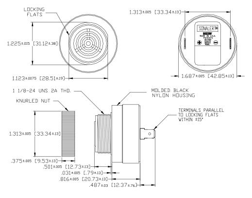
NDTE: MOUNTING- REMOVE BLACK PLASTIC NUT AND INSERT THREADED FRONT THROUGH 1.25" HOLE PUNCHED IN PANEL, IF ORIENTATION IS NEEDED, NOTE LOCKING FLATS ON DRAWING, SCREW NUT BACK ON. DO NOT OVERTIGHTEN.
