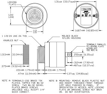
NOTE B: MOUNTING- REMOVE BLACK PLASTIC NUT AND INSERT THREADED FRINT THROUGH 1.25' HOLE PUNCHED IN PANEL, IF DRIENTATION IS NEEDED, NOTE LOCKING FLATS ON DRAVING. SCREW NUT BACK ON. DO NOT OVERTIGHTEN.
