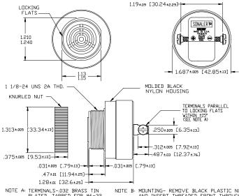
NOTE A: TERMINALS-0.32 BRASS TIN PLATED, TAPPED FIR #6-32 SCREW, TWD #6-32 NICKEL PLATED BRASS SCREWS INCLUBED, WILL ACCEPT 1/4' QUICK CONNECT. NOTE B: MOUNTING- REMOVE BLACK PLASTIC NUT AND INSERT THREADED FRONT THROUGH 1.25' HOLE PUNCHED IN PANEL, IF DRIENTATION IS NEEDED, NOTE LOCKING FLATS ON DRAWING. SCREW NUT BACK ON. DO NOT OVERTIGHTEN.
