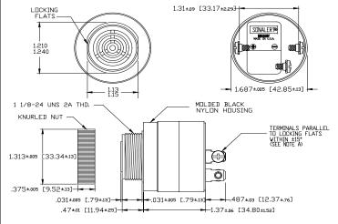
NOTE A: TERMINALS-.032 BRASS TIN PLATED, TAPPED FOR #6-32 SCREW. TWO #6-32 NICKEL PLATED BRASS SCREWS INCLUBED. WILL ACCEPT 1/4' QUICK CONNECT. NOTE B: MOUNTING- REMOVE BLACK PLASTIC NUT AND INSERT THREADED FRINT THROUGH 1.25' HOLE PUNCHED IN PANEL, IF DRIENTATION IS NEEDED, NOTE LOCKING FLATS ON DRAWING. SCREW NUT BACK ON. DO NOT OVERTIGHTEN.
