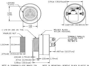
NOTE A TERMINALS-032 BRASS TIN PLATED, TAPPED FOR #6-32 SCREW. TWO #6-32 NICKEL PLATED BRASS SCREWS INCLUDED. WILL ACCEPT 1/47 QUICK CONNECT.
