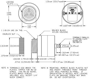
NOTE B: MOUNTING- REMOVE BLACK PLASTIC NUT AND INSERT THREADED FRONT THROUGH 1.25' HOLLE PUNCHED IN PANEL, IF ORIENTATION IS NEEDED, NOTE LOCKING FLATS ON DRAWING SCREW NUT BACK DO NOT OVERTIGHTEN.
