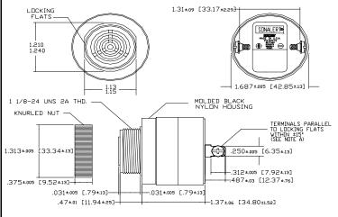
NOTE A: TERMINALS-.032 BRASS TIN PLATED, TAPPED FOR #6-32 SCREW. TWD #6-32 NICKEL PLATED BRASS SCREWS INCLUBED. WILL ACCEPT 1/4\* QUICK CONNECT.
