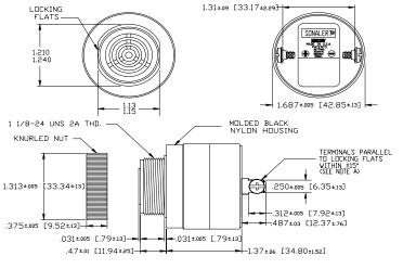
NOTE A: TERMINALS-.032 BRASS TIN PLATED, TAPPED FOR #6-32 SCREW. TWO #6-32 NICKEL PLATED BRASS SCREWS INCLUDED. VILL ACCEPT 1/4\* QUICK CONNECT.
