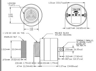
NOTE AF TERMINALS-.032 BRASS TIN PLATED, TAPPED FOR #6-32 SCREW. TWO #6-32 NICKEL PLATED BRASS SCREWS INCLUBED. WILL ACCEPT 1/4' QUICK CONNECT. NOTE B: MOUNTING- REMOVE BLACK PLASTIC NUT AND INSERT THREADED FRONT THROUGH 1.25' HOLE PUNCHED IN PANEL, IF DRIENTATION IS NEEDED, NOTE LOCKING FLATS ON DRAVING. SCREW NUT BACK ON. DO NOT DVERTIGHTEN.
