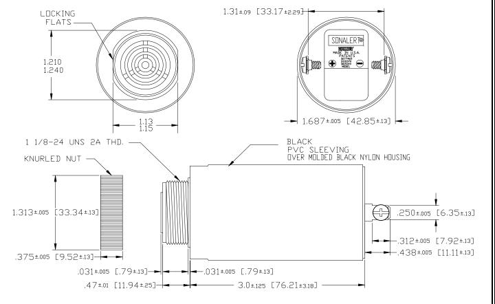
NOTE A: TERMINALS-.032 BRASS TIN PLATED, TAPPED FOR #6-32 TWO #6-32 NICKEL PLATED BRASS SCREWS INCLUDED. WILL ACCEPT 1/4" QUICK CONNECT.
