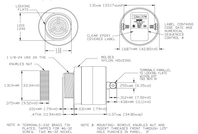
HOLE PUNCHED IN PANEL, IF ORIENTATION IS NEEDED, NOTE LOCKING
