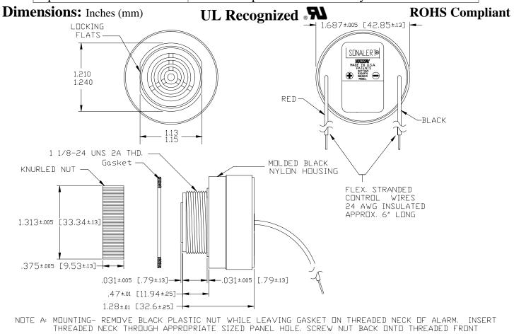
SECURING ALARM TO PANEL. MAX RECOMMENDED TORQUE IS 10 IN-LBS.
