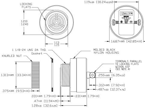
NOTE A: TERMINALS-.032 BRASS TIN PLATED, TAPPED FOR #6-32 SCREW. TWO #6-32 NICKEL PLATED BRASS SCREWS INCLUDED. WILL ACCEPT 1/4" QUICK
