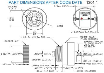
NOTE AF TERMINALS-0.32 BRASS TIN PLATED, TAPPED FOR #6-32 SCREW. TWO #6-32 NICKEL PLATED BRASS SCREWS INCLUDED. WILL ACCEPT 1/4' QUICK CONNECT. NOTE B: MOUNTING- REMOVE BLACK PLASTIC NUT AND INSERT THREADED FRONT THROUGH 1.25' HOLE PUNCHED IN PANEL, IF DRIENTATION IS NEEDED, NOTE LOCKING FLATS ON DRAWING. SCREW NUT BACK ON. DO NOT OVERTIGHTEN.
