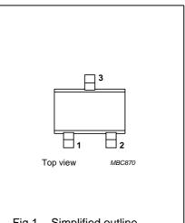
Fig.1 Simplified outline SOT323 and pin configuration.
