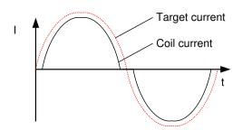
Coil current does not have optimum shape
