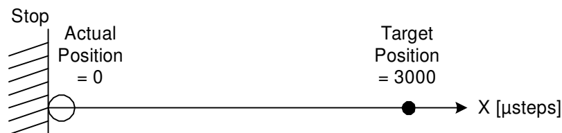
Figure 23: Positioning Example: Situation after reference search
