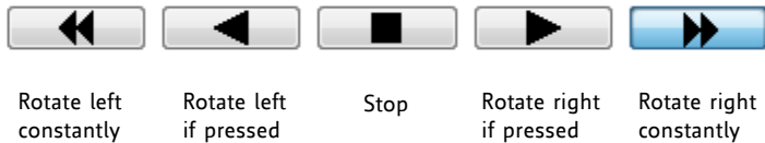
Figure 6.4 Jog tab keys for moving a motor
