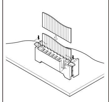
The FDZ connector, a Zero Insertion Force (ZIF) connector, was developed to connect FPC and membrane switch leads. This combination of features allows greater freedom in internal wiring designs. No force is required to insert the leads. Once inserted, the leads are securely held and locked by moving the slide. The contact is double-sided to ensure greater reliability.
