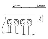
Note: 1. The above figure is the figure viewed from soldering side. 2. Tolerances are non-cumulative: ±0.05mm for all centers. \*Type A 0.8<sup>+0.1</sup><sub>-0.05</sub> dia. \*Type B 2 to 7 circuits: 0.75 ±0.05 dia.
