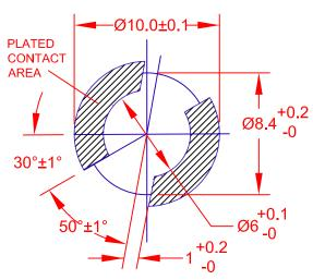
PC BOARD PUNCH PATTERN (NO TREATMENT, SUCH AS APPLICATION OF FLUX, SHALL BE DONE.)
