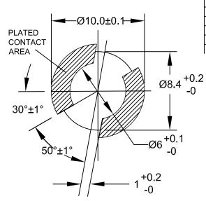
PC BOARD PUNCH PATTERN (NO TREATMENT, SUCH AS APPLICATION OF FLUX, SHALL BE DONE.)
