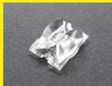
15.4mm X 19.6 mm PMMA
