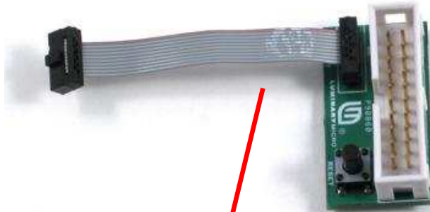
Figure 7 10-pin to 20-pin JTAG Adapter Module (P/N: MDL-ADA2)
