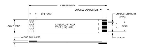
CABLE WIDTH = (# OF CONDUCTORS + 1)(PITCH)
