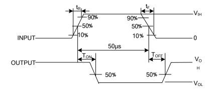
Note 1: Pulse width 50 $\mu$ s ,duty cycle 10% Output impedance 50 $\Omega$  t<sub>R</sub> 5ns, t<sub>F</sub> 10ns
