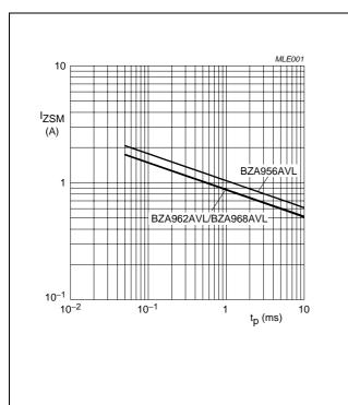
Fig.2 Maximum non-repetitive peak reverse current as a function of pulse time.
