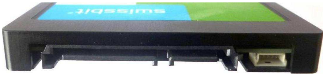
Figure 2: SSD connector side with power, SATA and feature connector
