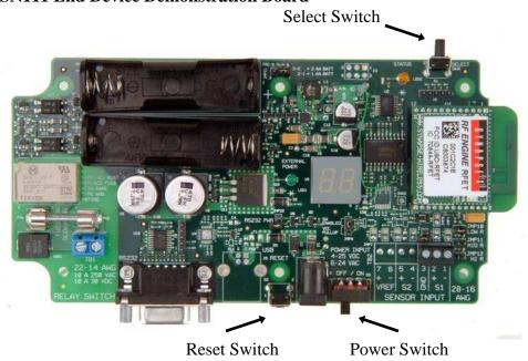
The Synapse SN111 End Device Demonstration Board features a push-button switch, LED, seven-segment display (two seven-segment digits, 14 segments total), and a generic sensor input.
