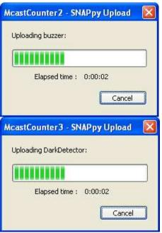
Select the "buzzer.py" example, and press OK (or you could double-click on the script name). Upload of the new SNAPpy Image (over the air!) should complete in a few seconds. The node will automatically restart when the upload finishes. (Depending on the script loaded into a node, restarting may not cause any visual change. In this case, the yellow LED will begin blinking after the node restarts. This node is the SNAP Engine on the SN171 Proto Board.)
