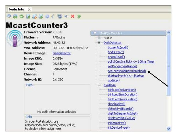
Notice the setThreshold() function. The script defaults to "beeping" when the darkness level crosses 85%, but you can change this threshold "on the fly" by calling this function.
