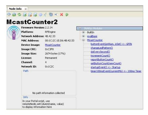
On the left-hand side, the Firmware Version, Platform, Network Address, MAC Address, Device Image, Image CRC, Image Size, License, Channel, and Network Id are shown. Below that is a block where Path information (the path to/from the node) can be displayed. Below that there is an Info field that can be controlled from Portal scripts to add your own custom field(s) to the Node Info panel.
