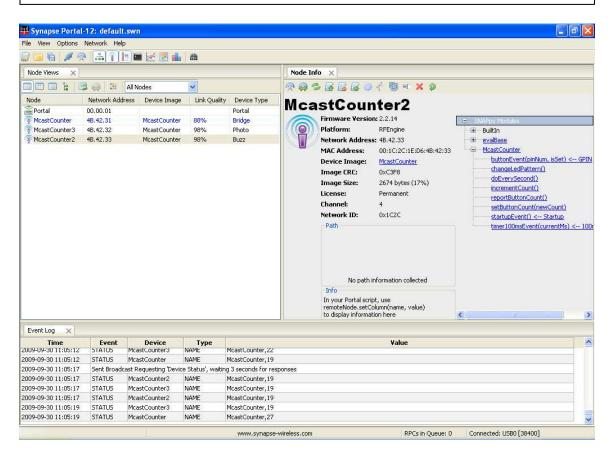
Note that the node names are based on the names of the SNAPpy scripts loaded into those same nodes *at the time of discovery*, but with additional trailing digits (2, 3, 4) added to enforce uniqueness.
