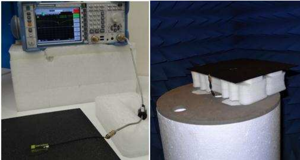
Figure 1: Impedance, isolation and correlation coefficient measurements (left hand) and peak gain, average gain, efficiency and radiation pattern measurements (right hand)
