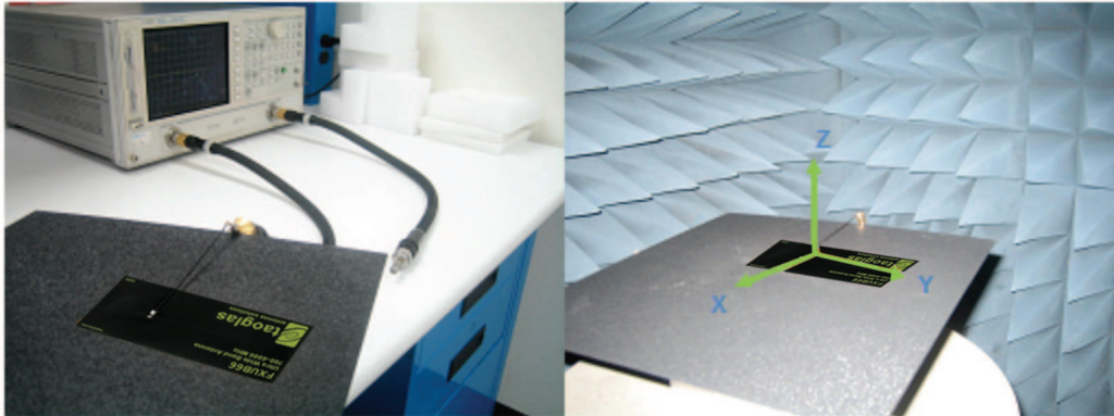
Figure 1. Impedance measurements (left hand) and peak gain, average gain, efficiency and radiation pattern measurements (right hand).
