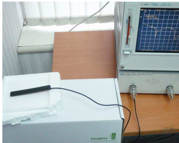
Free space Return Loss measurement setup
