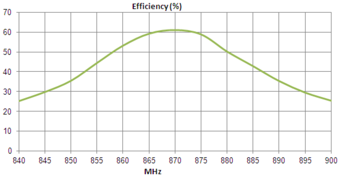
Figure 4. Efficiency of 868 MHz ISM Band Antenna ILA.02
