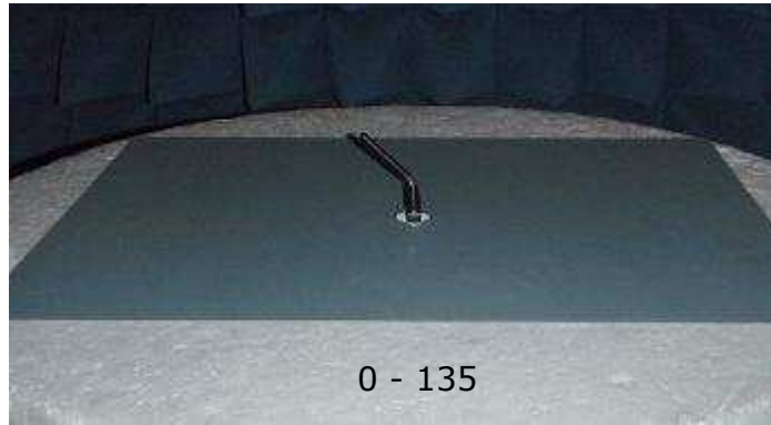
Example of TG.09 mounting on metal plane.
