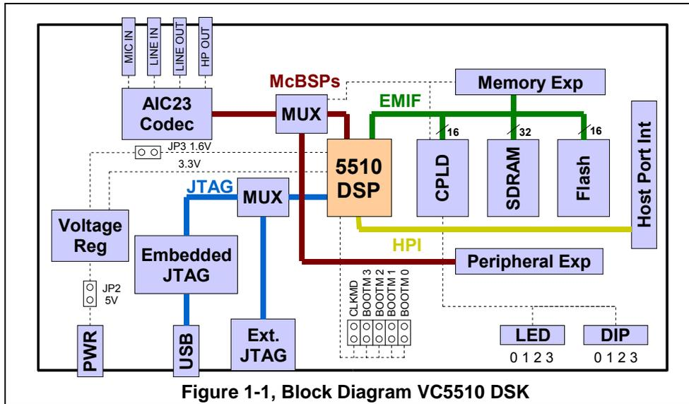
Figure 1-1, Block Diagram VC5510 DSK
