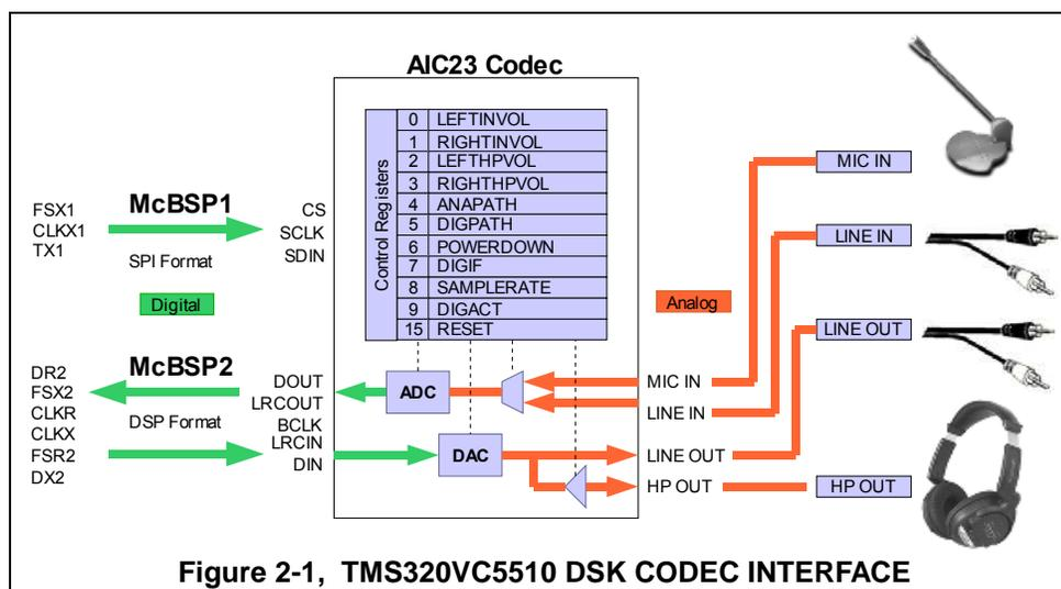
Figure 2-1, TMS320VC5510 DSK CODEC INTERFACE
