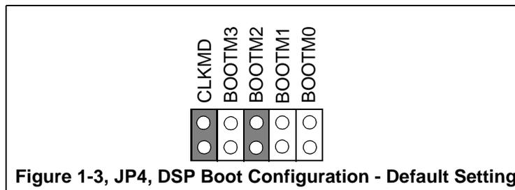
The jumpers drive signals that directly correspond to the input on one of the DSP's configuration pins. If the jumper is on, the signal is driven to a logic 0. If the jumper is off, the signal is driven to a logic 1.
