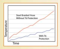
When applied, the aluminum laminate reflects heat away and the insulating fiberglass backing protects the fragile contents from thermal damage and failure. T6 can reduce the heat transmission from hot pipes or engine components into hoses or harnesses by up to 50% or more.
