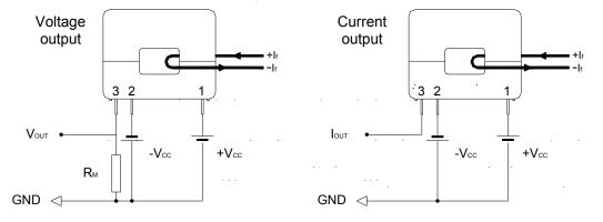
$\begin{array}{l} \text{S25P100D15X} \\ \text{At I}_{\text{f}} = 100\text{A \& V_{\text{CC}} = \pm 15V_{\text{DC}} \\ \text{40}\Omega \leq R_{\text{M}} \leq 95\Omega \end{array}$
