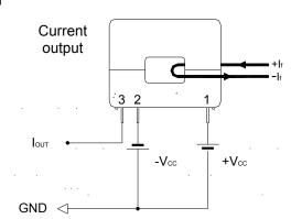
S25P100D15YAt  $I_f = 100A \& V_{CC} = \pm 15V_{DC}$  $20Ω \le R_M \le 102Ω$
