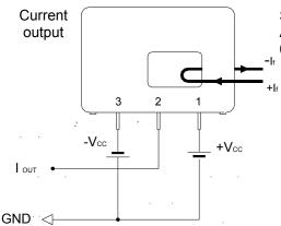
S26P200D15Y At  $I_f$  = 200A &  $V_{CC}$  = ±15 $V_{DC}$ 0Ω ≤  $R_M$  ≤ 56Ω
