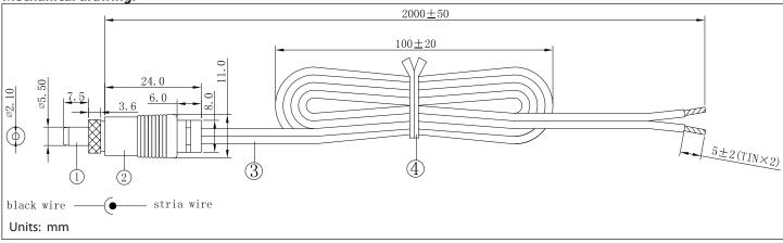
**tolerance** X: ±0.5 mm .X: ±0.3 mm .XX: ±0.05 mm applicable unless otherwise indicated in specification or on drawings Tensility International Corporation reserves the right to substitute parts which are functionally equivalent to the ones specified.
