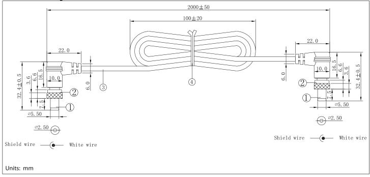
**tolerance** X: ±0.5 mm .X: ±0.3 mm .XX: ±0.05 mm applicable unless otherwise indicated in specification or on drawings Tensility International Corporation reserves the right to substitute parts which are functionally equivalent to the ones specified.
