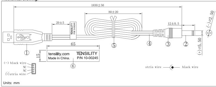
**tolerance** X: ±0.5 mm .X: ±0.3 mm .XX: ±0.05 mm applicable unless otherwise indicated in specification or on drawings Tensility International Corporation reserves the right to substitute parts which are functionally equivalent to the ones specified.
