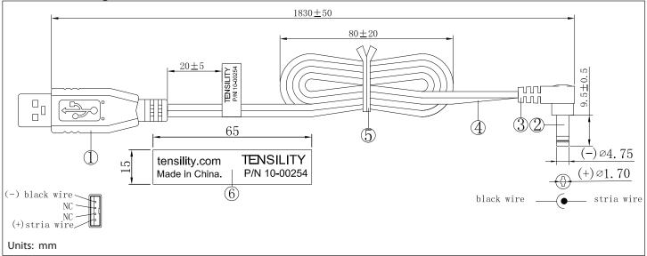
tolerance X: ±0.5 mm .X: ±0.3 mm .XX: ±0.05 mm applicable unless otherwise indicated in specification or on drawings Tensility International Corporation reserves the right to substitute
