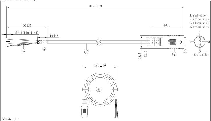
**tolerance** X: ±0.5 mm .X: ±0.3 mm .XX: ±0.05 mm applicable unless otherwise indicated in specification or on drawings Tensility International Corporation reserves the right to substitute parts which are functionally equivalent to the ones specified.
