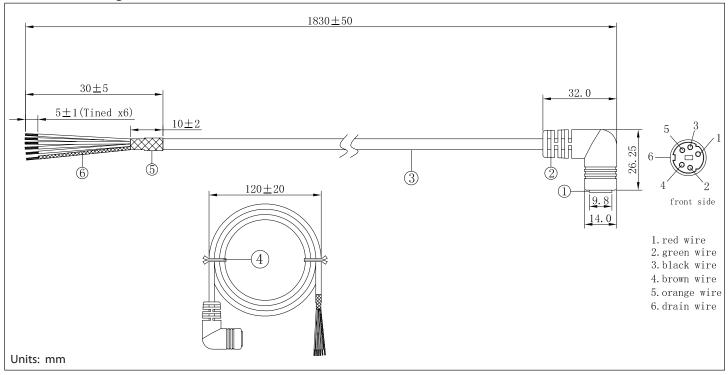
**tolerance** X: ±0.5 mm .X: ±0.3 mm .XX: ±0.05 mm applicable unless otherwise indicated in specification or on drawings Tensility International Corporation reserves the right to substitute parts which are functionally equivalent to the ones specified.
