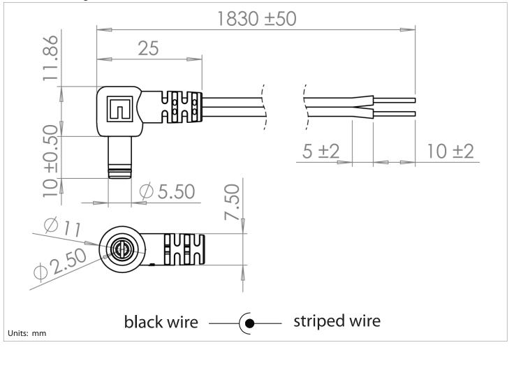
tolerance X: ±0.5 mm .X: ±0.3 mm .XX: ±0.05 mm applicable unless otherwise indicated in specification or on drawings Tensility International Corporation reserves the right to substitute parts which are functionally equivalent to the ones specified.
