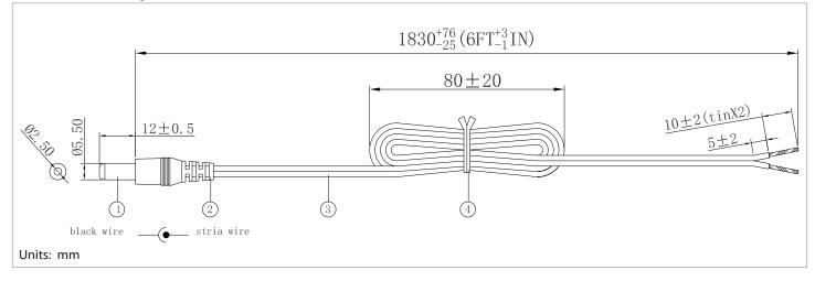
tolerance X: ±0.5 mm .X: ±0.3 mm .XX: ±0.05 mm applicable unless otherwise indicated in specification or on drawings
