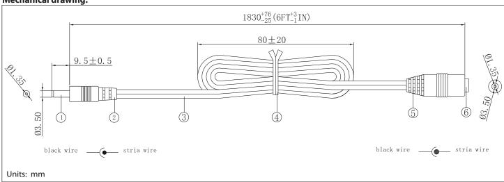
tolerance X: ±0.5 mm .X: ±0.3 mm .XX: ±0.05 mm applicable unless otherwise indicated in specification or on drawings Tensility International Corporation reserves the right to substitute parts which are functionally equivalent to the ones specified.
