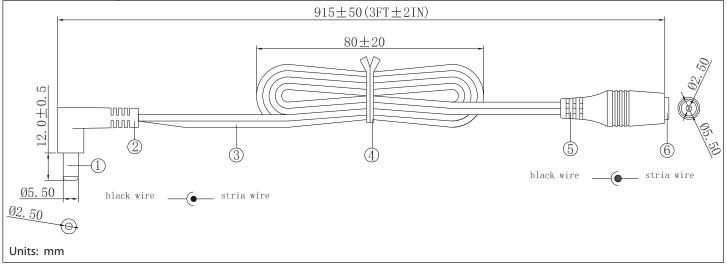
tolerance X: ±0.5 mm .X: ±0.3 mm .XX: ±0.05 mm applicable unless otherwise indicated in specification or on drawings Tensility International Corporation reserves the right to substitute
