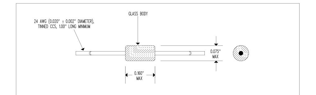
RESISTANCE @  $+25^{\circ}C = 2,000 \ \Omega \pm 10^{\circ}$ RESISTANCE/TEMPERATURE CURVE = "F"
